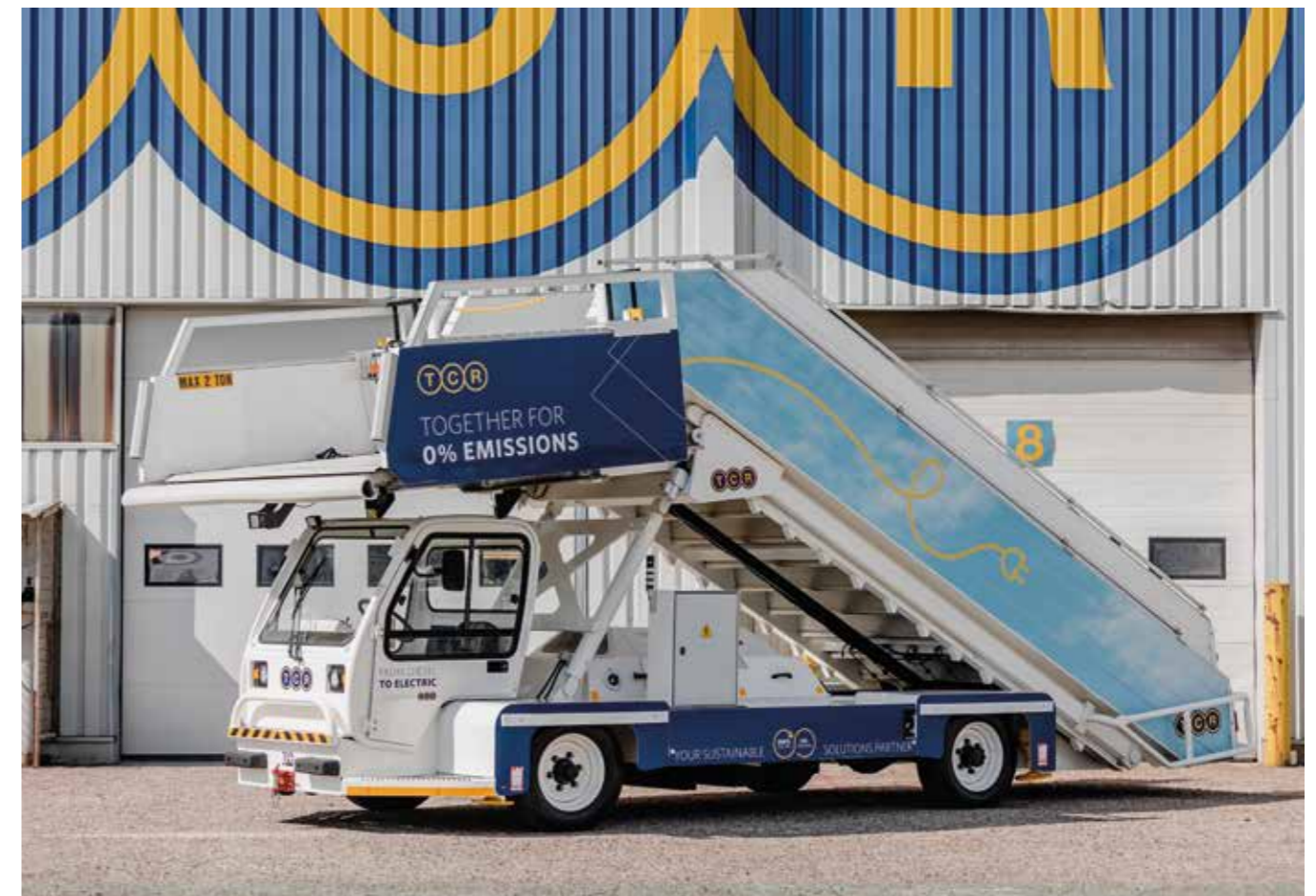
Example: Conversion of ABS 580 steps in cooperation with Interappra at TCR facility in Manchester
